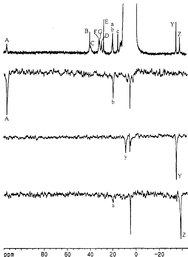
Figure 7. ^1\text{H} NMR spectra (600 MHz, 298 K) of an approximately 50/50 mixture of oxidized and reduced forms of 4 : upper trace, reference spectrum; lower traces, saturation transfer experiments establishing the correspondences of hyperfine shifted signals in the oxidized and reduced form of 4 . The correspondences A–b, Y–y and Z–a are presented.
